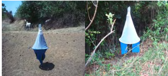
a) Challier / Laveissière trap b) Vavoua mono conical trap Photo: Dao Balabadi Photo: Dao Balabadi
